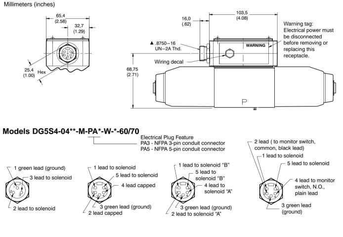
▲ Electrical connection is over solenoid on single solenoid models, and over "b" solenoid on dual solenoid models. See diagram plate for "b" solenoid location. Electrical rating 600 volts, 3 pole, 10 amps and 5 pole, 8 amps. The female portable plug to be furnished by customer.
