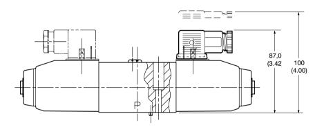
Connector can be positioned at  $90^{\circ}$  intervals on valve by re-assembling contact holder into appropriate position inside connector housing.
